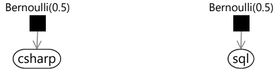
Figure 2.2: Factor graph showing priors for the binary skill variables csharp and sql .
